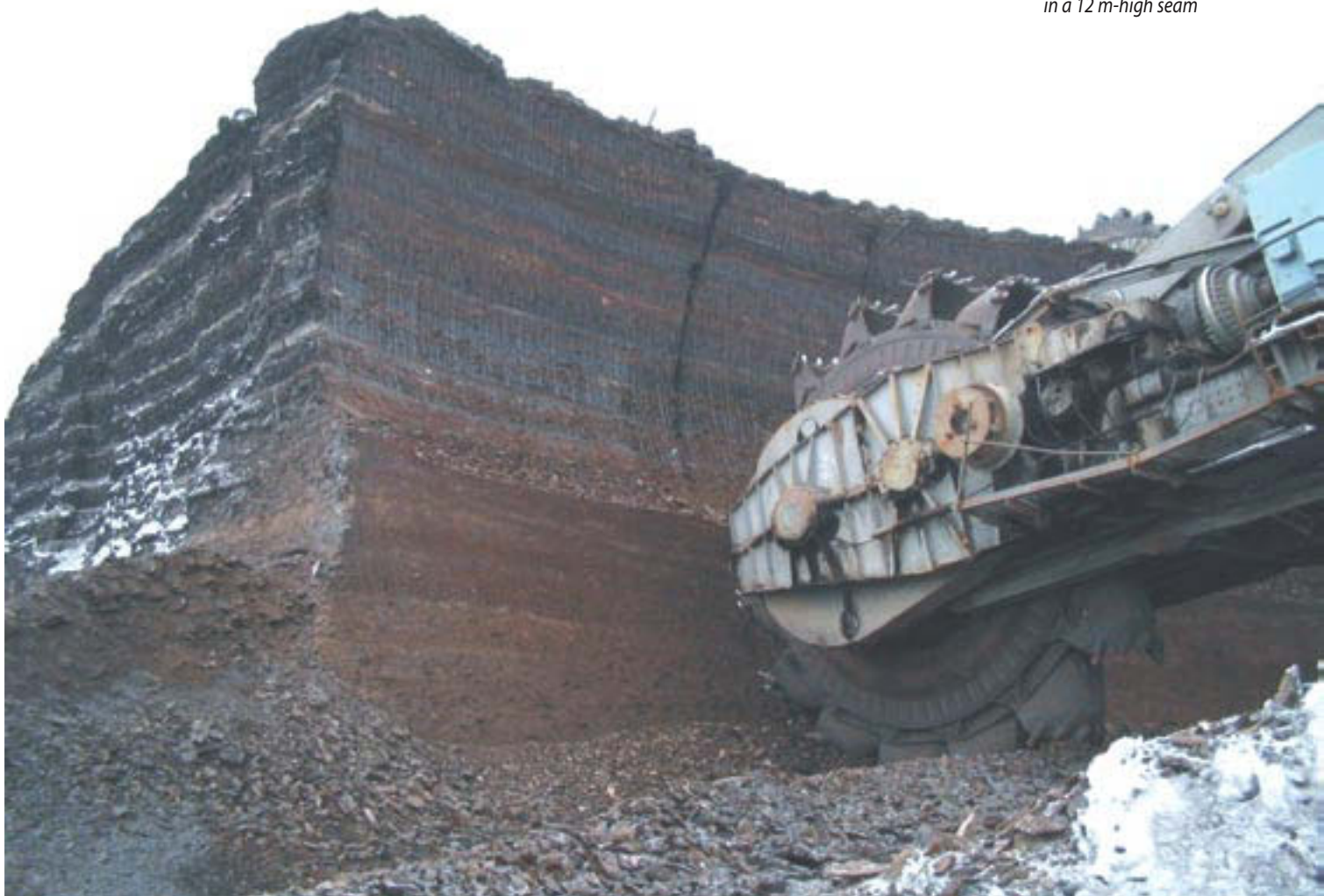
Bucket-wheel excavator exploiting lignite in a 12 m-high seam
