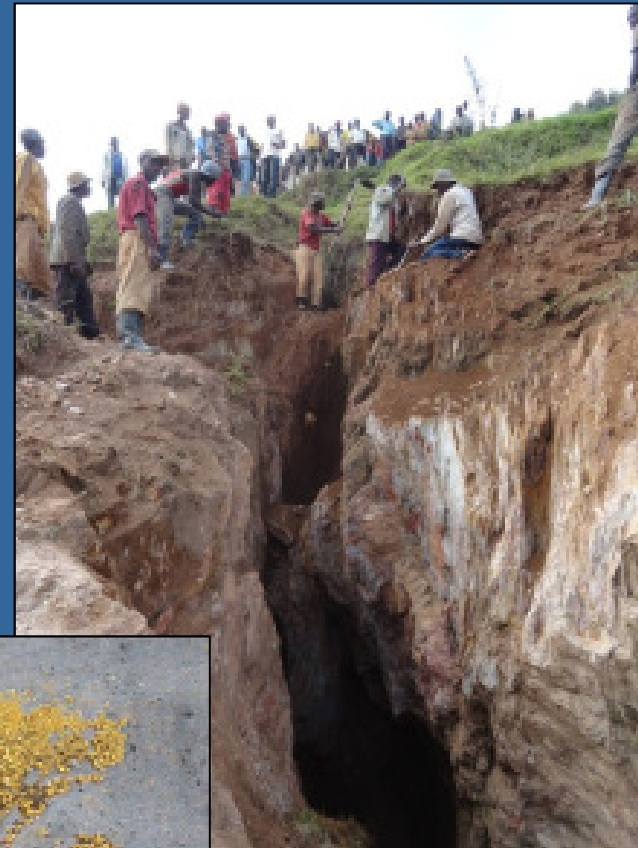
Au-Mineralisation in Quartz-Veins, Miyove/ Rwanda
